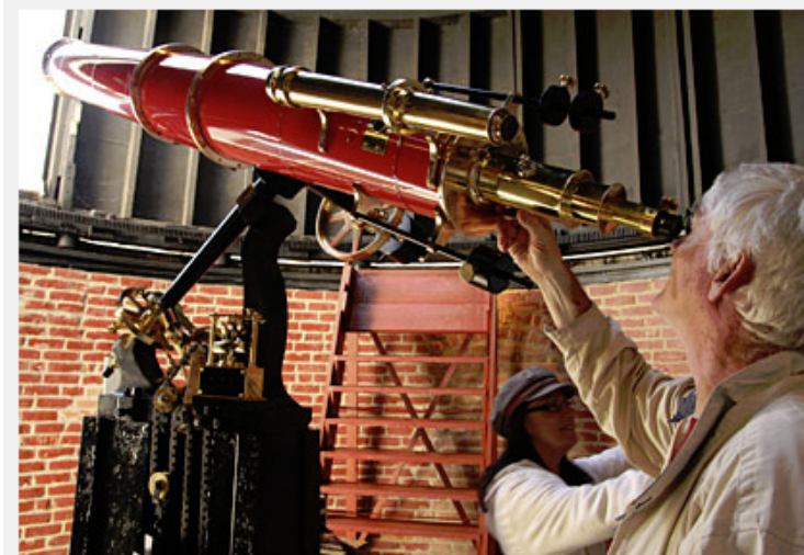
The Seagrave 8-inch Clark refractor, in like-new condition after 134 years.
